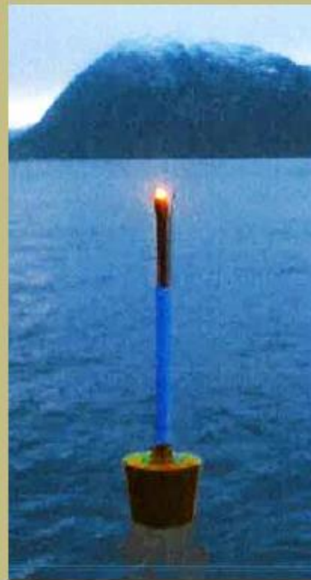
Light marked buoy with linear generator
