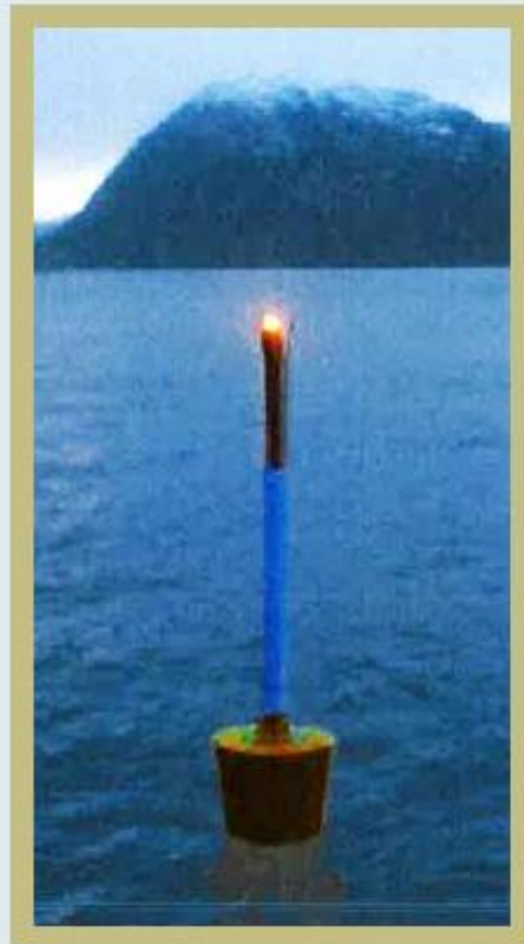
Light marked buoy with linear generator
