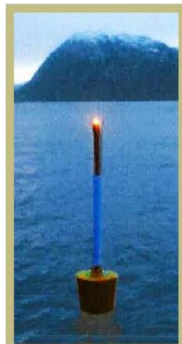
Light marked buoy with linear generator
