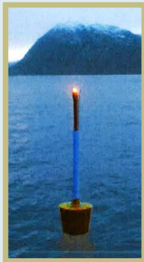
Light marked buoy with magnet generator
