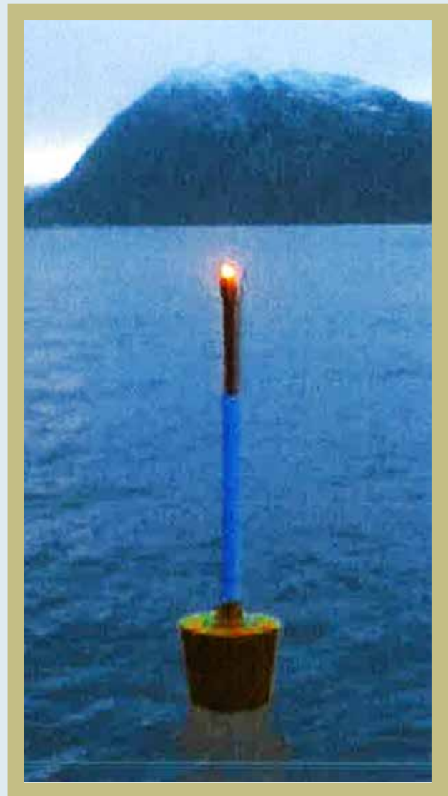
Light marked buoy with magnet generator
