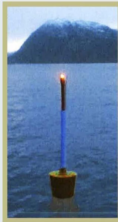
Light marked buoy with magnet generator
