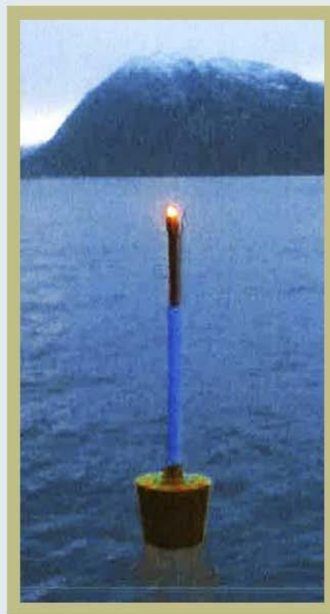
Light marked buoy with magnet generator
